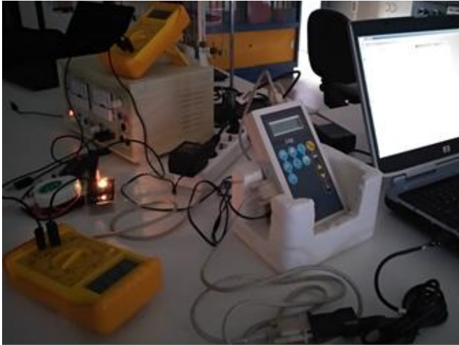
Figure 2. Experimental setup to measure the emitted power of an incandescent lamp, by calculating filaments' temperature of the lamp.
