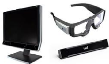
Fig. 2. Basic equipment setup of an eye tracking laboratory space
