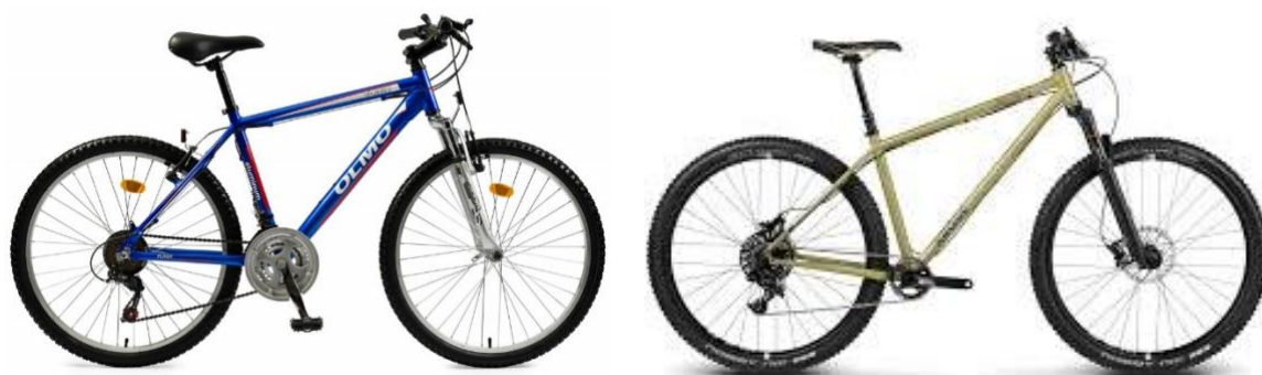
Figure 1. Steel (option A) and aluminium (option B) frame bicycle
